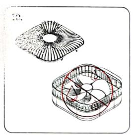
Disassemble the detachable cover to clean the dust. Use dry cloth to wipe the fan body, forbidden to wash with water.
