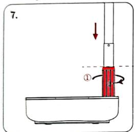
Folding 1:Please turn the handle device clockwise to unlock.
