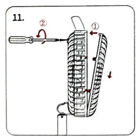
Align the clip position and tighten the screws to mount it back after the fan cover was dried.
