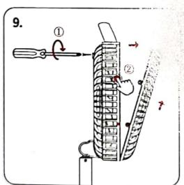
①Remove two screws on the top of the fan. ②Press side release clips to release the fan cover.
