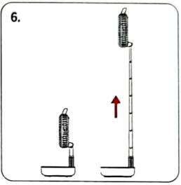
It provides adjustable height to meet variable need. Please pull the rod up and down gently while adjusting to your preferred height.
