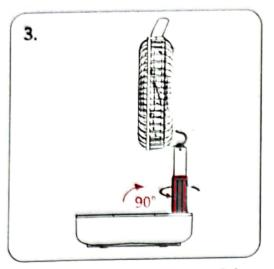
Turn the angle to 90° vertical, and then anticlockwise lock the handle device to fix the angle after unfolding the fan.
