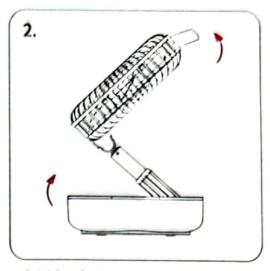
Unfold fan following the arrow direction.
